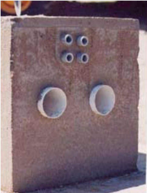
Figure 2. Flowable Fill Dry
